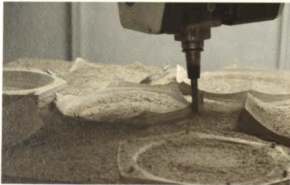
等待五轴CNC铣削加工的能组合成理想几何体的粗略聚合构件（上图）。密歇根大学建筑与城市规划学院FABLab工作室的建造支持（下图）。Roughed aggregated blanks of the desired geometry await the milling operation on the five-axis machine (above). With fabrication support by the University of Michigan Taubman College FABLab (below).
