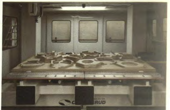
等待五轴CNC铣削加工的能组合成理想几何体的粗略聚合构件（上图）。密歇根大学建筑与城市规划学院FABLab工作室的建造支持（下图）。Roughed aggregated blanks of the desired geometry await the milling operation on the five-axis machine (above). With fabrication support by the University of Michigan Taubman College FABLab (below).
